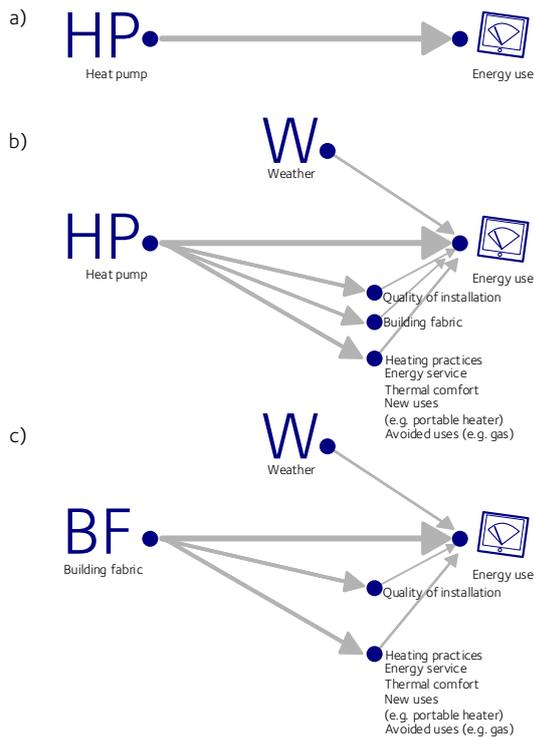
Figure 5: Causal models for the impact of heat pumps on energy use
