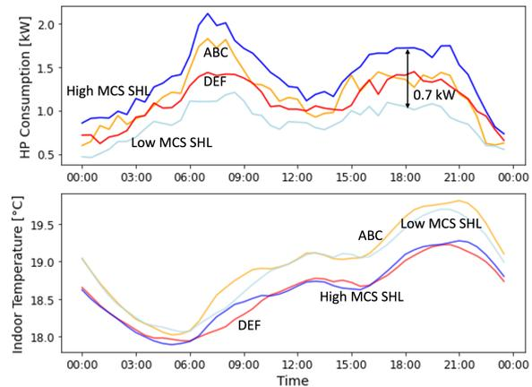
Figure 6: Causal (?) difference between homes with high and low heat loss. Source: Perelli-Rocco (2023)
